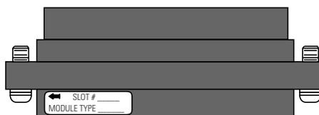
To remove the terminal block, loosen the upper and lower retaining screws. The terminal block will back away from the module as you remove the screws. When replacing the terminal block, torque the retaining screws to 0.46 Nm (4.1 in-lbs).
