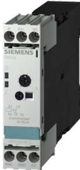
Timing relay, electronic Phase-out product! For further information, contact our sales department ON delay 1 CO contact 15 time ranges 0.05 s...100 h 24, 200...240 V AC and 24 V DC at 50/60 Hz AC with LED, screw terminal
