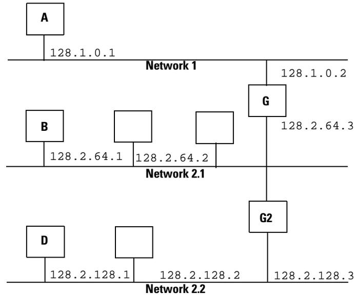
A second network with Hosts D and E was added. Gateway G2 connects Network 2.1 with Network 2.2.
