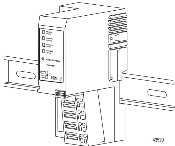
1. Position the adapter vertically above the DIN rail.
