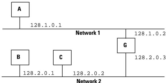
When host B with IP address 128.2.0.1 communicates with host C, it knows from C's IP address that C is on the same network. In an Ethernet environment, B can then resolve C's IP address into a hardware address (MAC address) and communicate with C directly.
